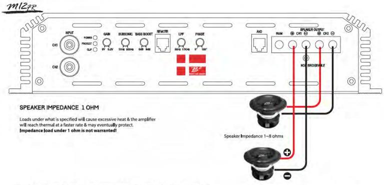
The M12FR can be used in a subwoofer or a full range speaker configuration.
