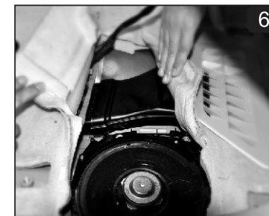
Loosen the 4 mounting screws of the carpet panel and remove it.
