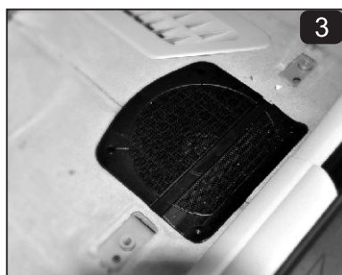
Factory subwoofer is under the cover, ready for the B2 audio BWF8 installation.
