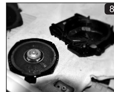
In case of the factory subwoofer is glued, be careful not to damage the plastic enclosure which can be re used for the B2 audio BWF8.
