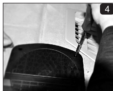
Loosen the factory fixed screws of the subwoofer cover.
