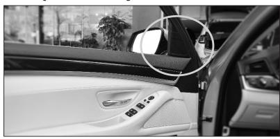
2. Carefully pry out the blank tweeter housing. (Before starting, we recommend to fully open the window, this will help during the operation)
