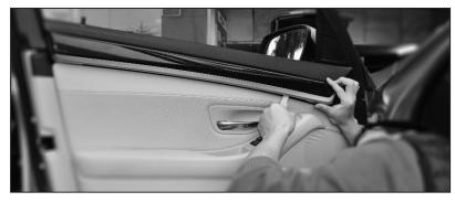
You will need to lift up the trim piece first and then slide outward to release the trim from the door panel, as seen in the below photo. (Red arrows.)
