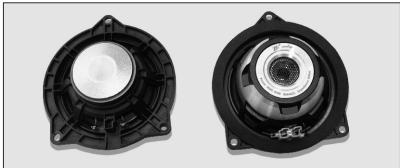
8. Replace the original mid-range speaker with B2 audio mid-range speaker, using the original bolts. Once the speaker mounting is done, reconnect the speaker wire and the provided crossover network&inline crossover. Then you have to fix the crossover network to the door panel (by using the double adhesive tape which is already attached on the crossover network or cable ties)
