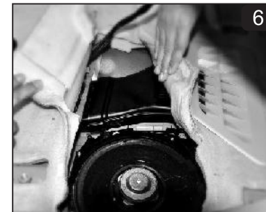
Loosen the 4 mounting screws of the carpet panel and remove it.
