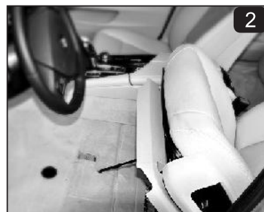
After the screws removal, tilt down the seat to provide access to the subwoofer replacement.
