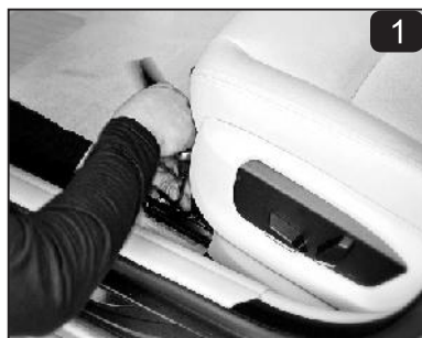
Remove the screws that hold the driver's seat track to the floor.
