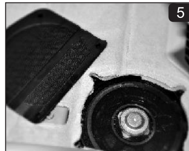
Once all the fixed screws are loosened, remove cover to expose factory subwoofer.
