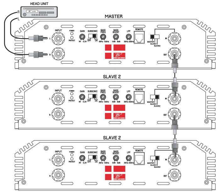
To link the master and slave 2 amplifiers in daisy chain mode follow the steps below. Each slave 2 will be controlled by the master's control panel, but the speakers must be connected individually to each amp. The daisy chain is a true benefit when you have multiple speakers and amps.
