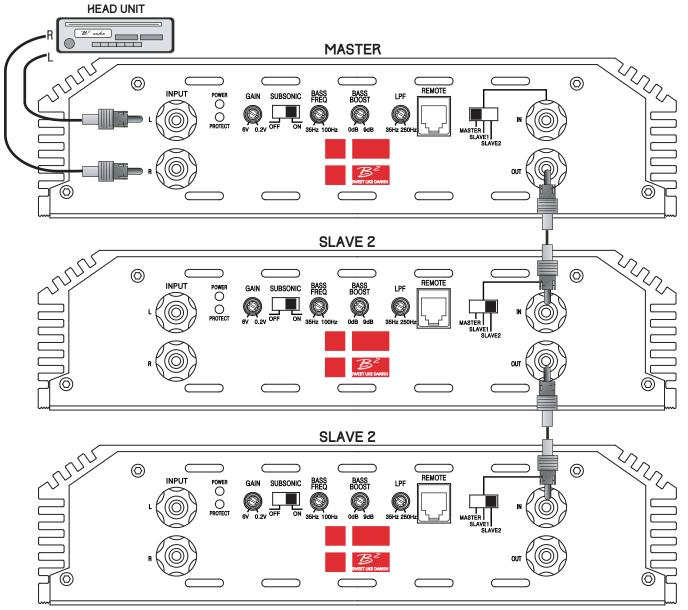
To link the master and slave 2 amplifiers in daisy chain mode follow the steps below. Each slave 2 will be controlled by the master's control panel, but the speakers must be connected individually to each amp. The daisy chain is a true benefit when you have multiple speakers and amps.
